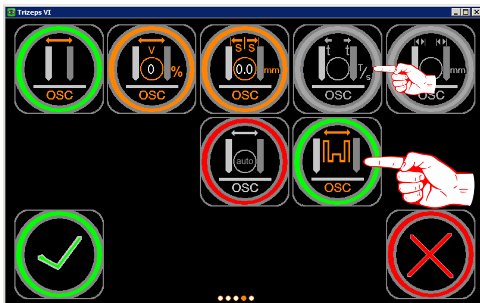
Picture 1 OSC Synchronization enabled, OSC Border Dwell Time automatically disabled
