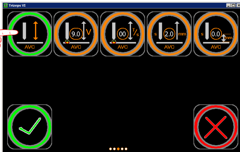
Picture 1 AVC activated (green button), simultaneously opens four additional buttons (orange) for further adjustment possibilities
